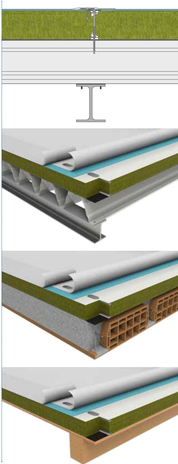
ISOFIRE WALL FLAT SYSTEM can be used for the composition of the ISODECK LG system, using Isopan corrugated metal sheets:
