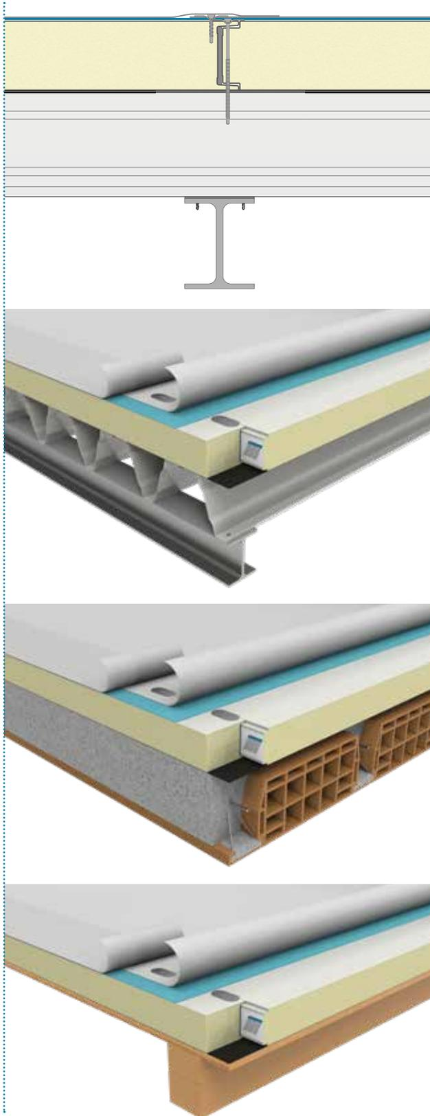
ISOPIANO FLAT SYSTEM can be used for the composition of the ISODECK LG system, using Isopan corrugated metal sheets:
