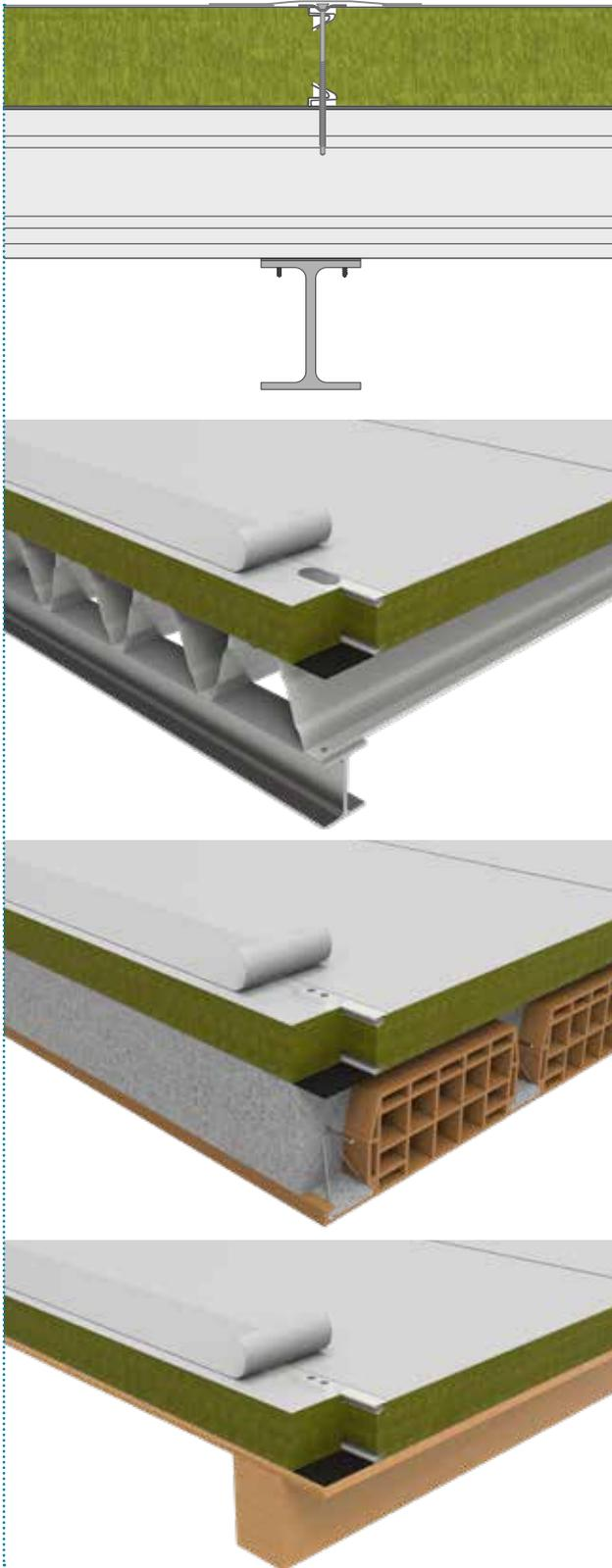
ISOFIRE WALL PVSTEEL can be used for the composition of the ISODECK LG system, using Isopan corrugated metal sheets:
